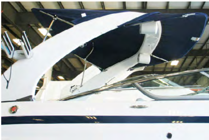
TYPICAL POWER TOWER- SUNSHADES IN CRUISE POSITION
