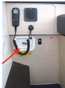
Ref 2: Remote pull switches Location: Steering station
