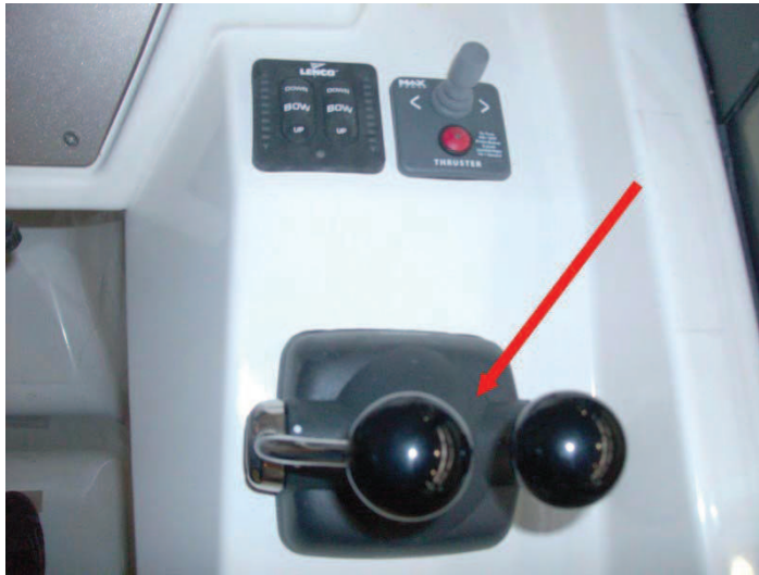
Engine control lever - Inside wheelhouse
