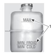
1. Level between marks when engine is B00067 cold
