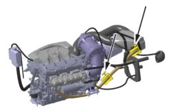
Rotax 4-TEC 250 ECT (requires 2) 1. Hose Pincher Tool, P/N 460717
