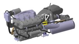
Rotax 4-TEC 200 ECT 1. Hose Pincher Tool, P/N 460717
