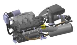
Rotax 4-TEC 150 1. Hose Pincher Tool, P/N 460717
