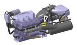
Rotax 4-TEC 250 1. Hose Pincher Tool, P/N 460717
