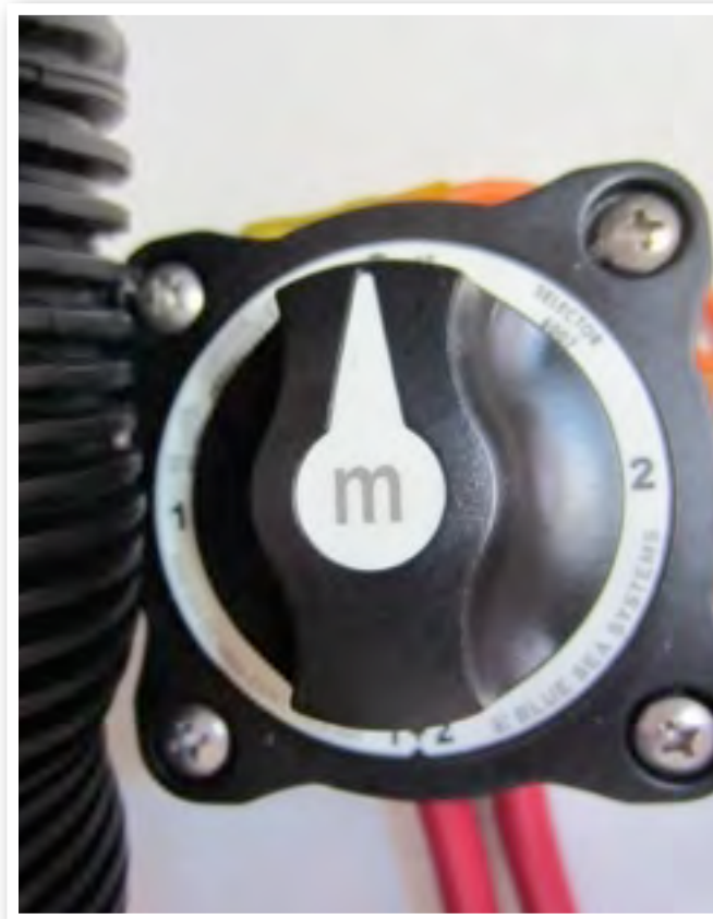
Battery Switch, Shown in the "Off" Position
