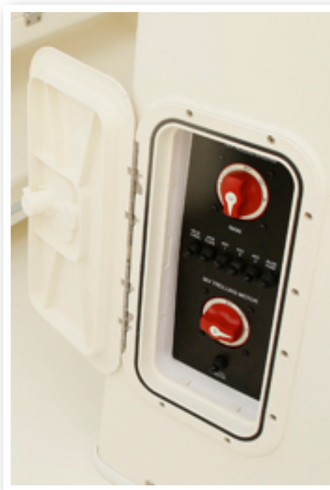
Battery Switch, Shown in the "Off" Position
