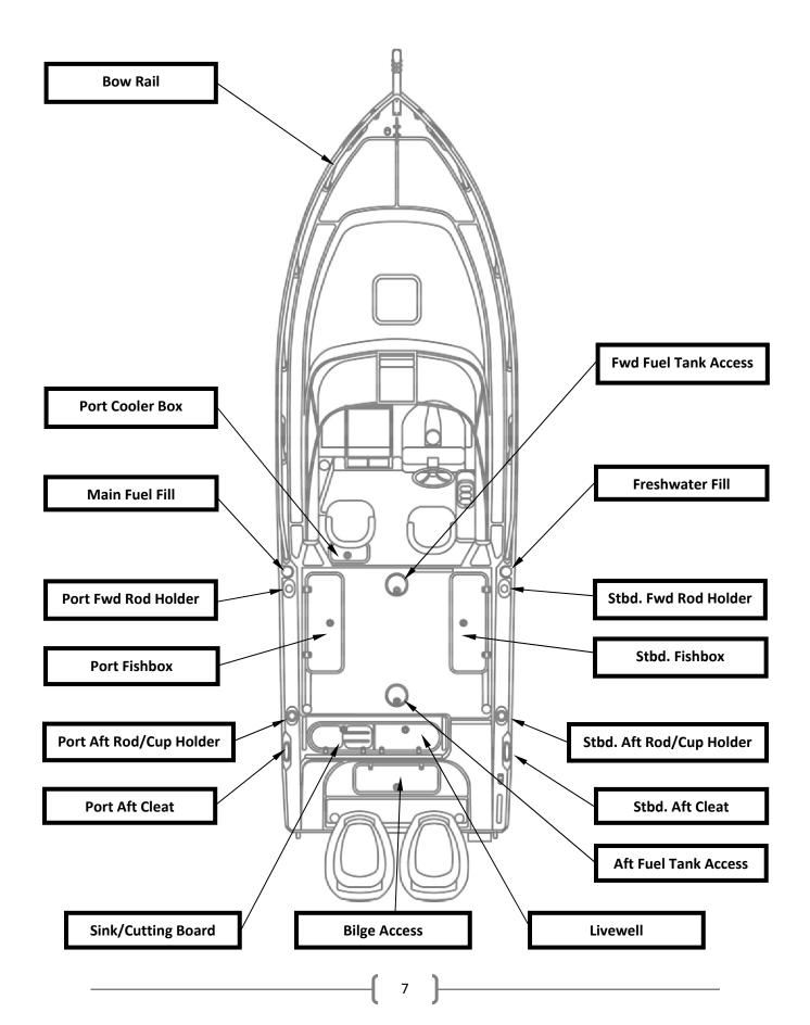
5b. Deck Layout: with bow rail removed for clarity.
