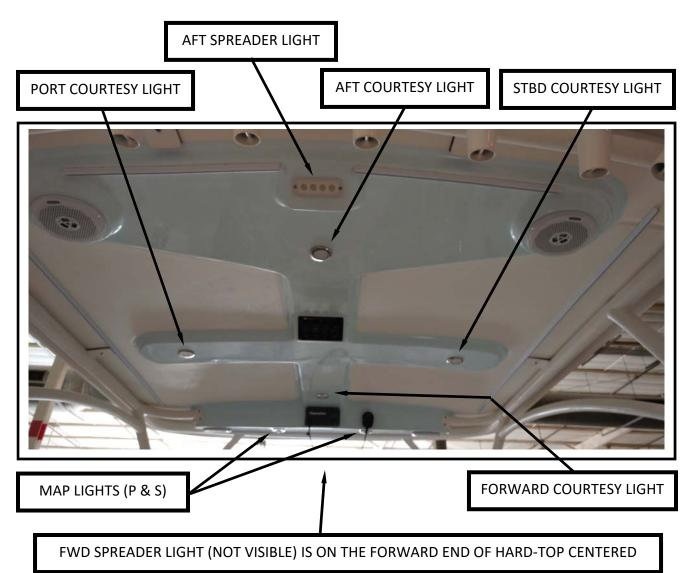
*Map lights*: There are two units located on the port and starboard underside of the forward raised portion of the hard-top, directly above the helm and the passenger console area.
