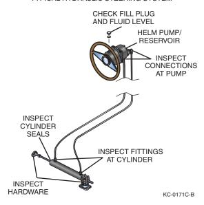
Make sure hydraulic hoses are tight and leak-free. Check cylinder seals for dampness, which indicates leaking. Check the fluid reservoir monthly and top off if necessary. See the steering system manufacturer's information for more details.
