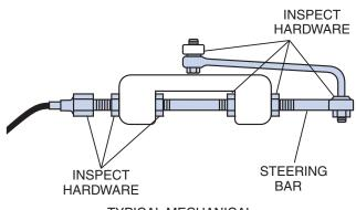
TYPICAL MECHANICAL OUTBOARD ENGINE STEERING LINK
