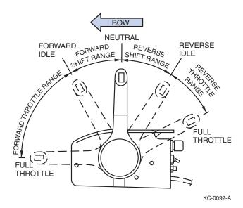
NEUTRAL - The lever is detented in the NEUTRAL position (center of travel) for starting; the neutral safety switch allows starting in this position only. For engine warm-up, a separate lever or button on the control is used to disengage the shift cable and allow the throttle to advance only while the transmission remains in NEUTRAL.
