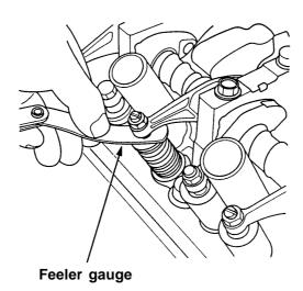
(10) Position the camshaft pulley to the top-dead-center points of compression stroke of other pistons, and repeat the steps (8) and (9).
