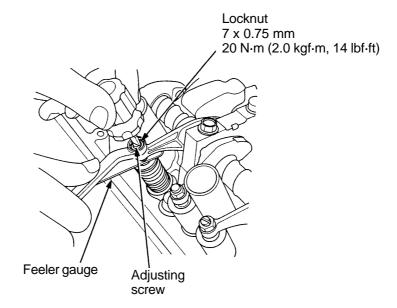
(9) Tighten the lock nut and measure the tappet clearance again with a feeler gauge.
