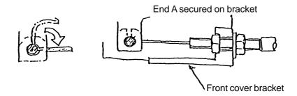
(3) Insert the hook of the cable extending from the end B of the cover lock cable B into the slot in the left side lock arm, fit the end B in the groove of the side cover bracket, then tighten the washer-attached nut to secure the end B on the bracket.
