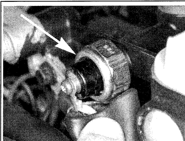
Fig. 237 Although oil pressure switch location varies slightly by model, it is always threaded into an oil passage on the powerhead
