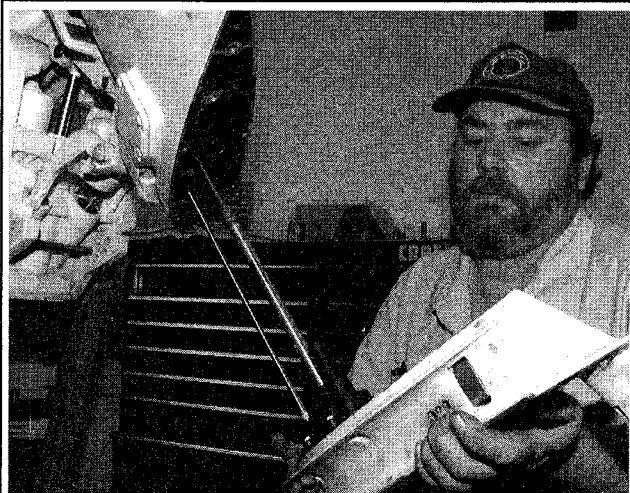
Fig. 33 ... and carefully lower the gearcase from the powerhead taking care not to damage the driveshaft, shift rod or water tube
