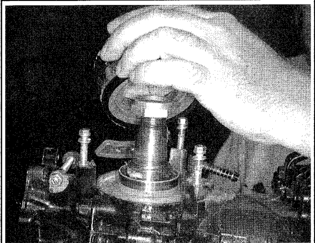
Fig. 80 ...then lift the timer base from the powerhead
