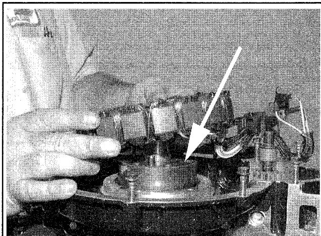
Fig. 86 ... or this timer base assembly found on some 25-55 hp (737cc) motors and all 25-70 hp (913cc) motors
