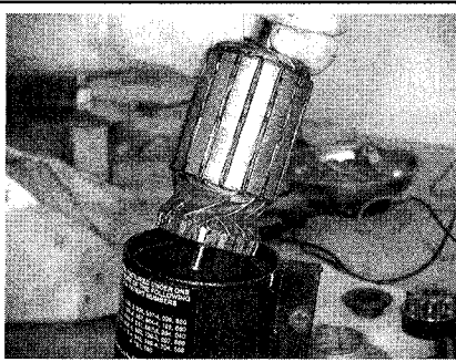
Fig. 208 Take care when inserting the armature in the starter housing, as permanent magnets will pull it inward strongly
