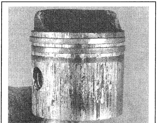
Fig. 1 Damaged piston, possibly caused by; using too-low an octane fuel; using fuel that had "soured" or by insufficient oil (in fuel on 2-strokes or in a crankcase on 4-strokes)
