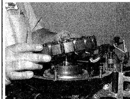
Fig. 60 . . . then lift the coil from the mounting plate
