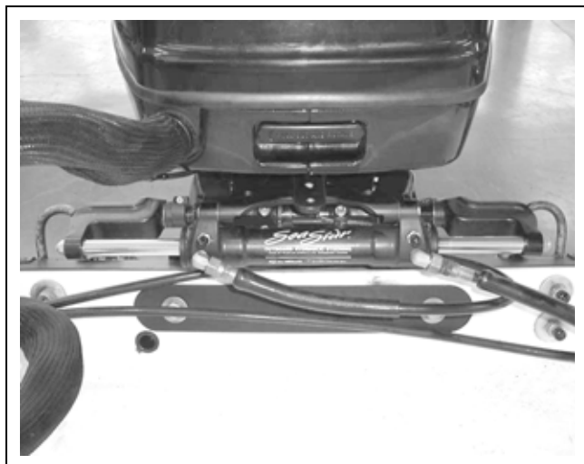
Typical manual hydraulic steering
