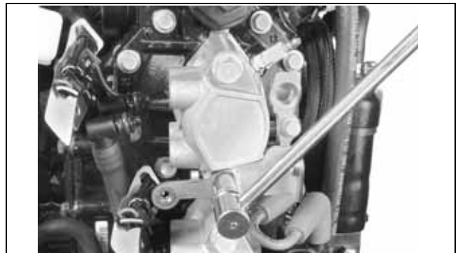
Tighten Screws in Stages
