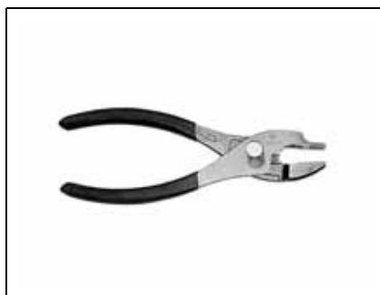
Installer, ball socket P/N 342225 002583
