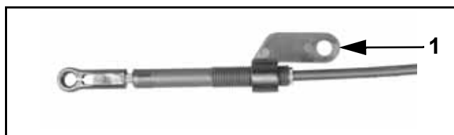
1. Turn anchor four turns toward cable end.
