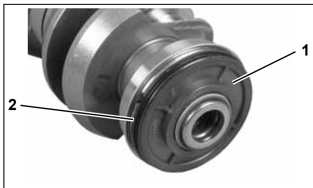
1. Lower seal housing 2. O-ring
