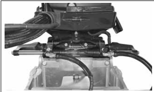
TYPICAL Manual Hydraulic Steering
