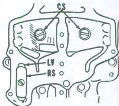
Fig. OM4-4—View of crankcase with intake manifold removed. The reed-type crankcase bleeder valve (LV) and stop (RS) can be removed for service, with manifold off. The two center main bearing screws (CS) must be removed before crankcase can be disassembled.
