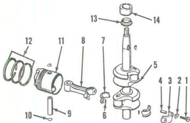
Fig. OM4-13—When attaching connecting rod to crankshaft, make certain that dowels (4) are positioned correctly and 30 bearing needles (6) are in each race. A lip type seal is used in place of slinger (13) on 1967 and late 1966 motors.
