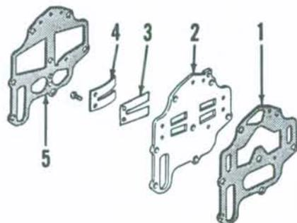
Fig. OM4-3—Exploded view of inlet leaf valve plate and associated parts.
