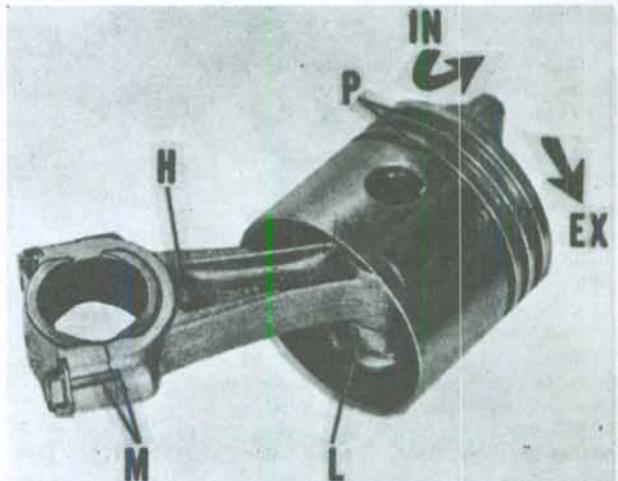
Fig. OM4-12 — Piston must be correctly assembled to rod with long, sloping side of piston head toward exhaust (EX) and oil hole (H) in rod up. When installing rod cap, make certain that marks (M) on rod and cap are aligned.
