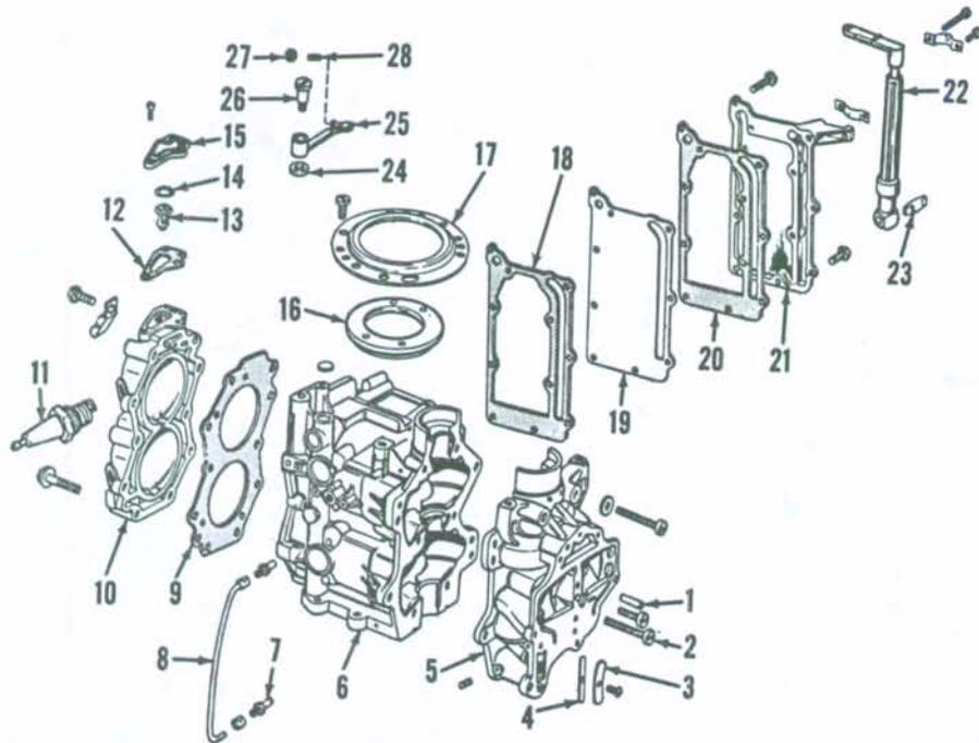
Fig. OM4-11—Exploded view of power head of the type used. Speed control lever (22 & 23) is used only on 6 hp models; armature detent (24 through 28) only on 5 hp units.
