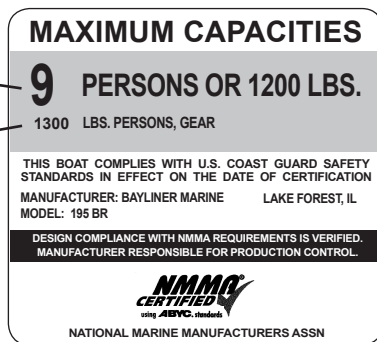
Capacity Plate (Domestic Certification)
